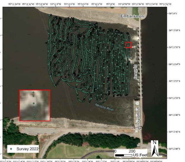
Figure 7d: Point distribution of 2022 bathymetry survey. Red box is magnified view of the datapoints taken during the survey.
