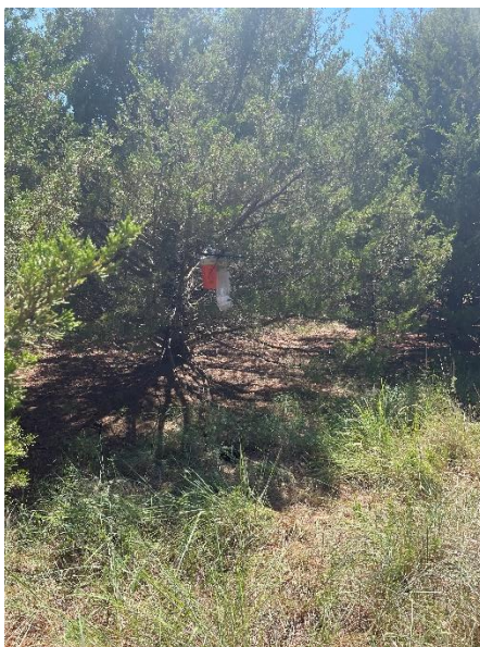
Figure A.2. CDC Light trap, without light, baited with two pounds of dry ice.
