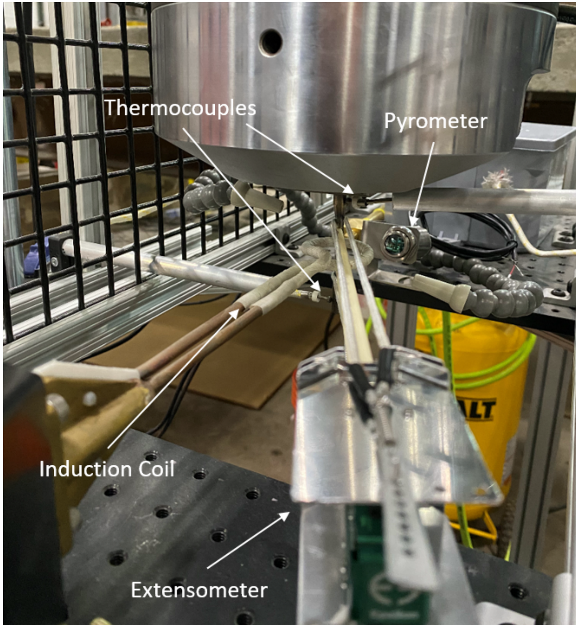
Figure III.2: Assembled Work Area Front View with INC718 Specimen
