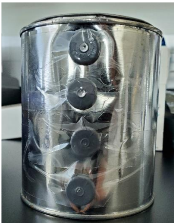
Figure 1. Headspace can with five sampling points at the rubber septa.
