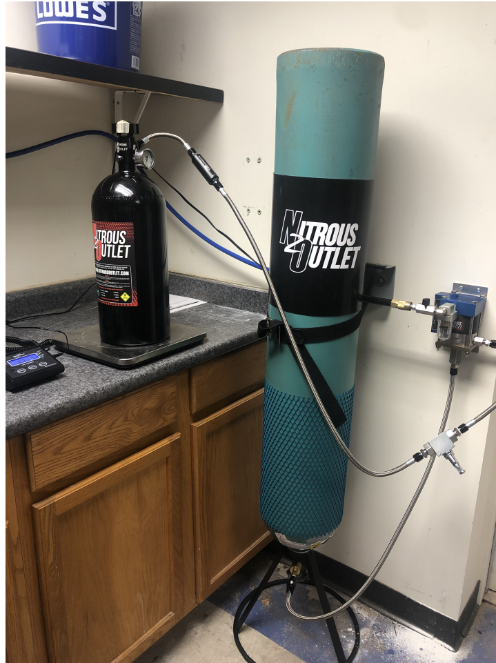
Figure 27: NOS Refill Station.
