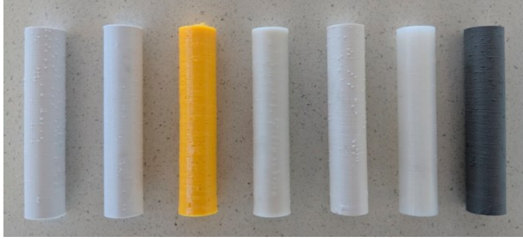
Figure 21: Small-scale fuel grains, left to right: ABS, PLA, PETG, PP, ASA, Nylon, and PLA with AL. [18]
