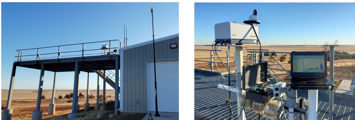
Figure 2.4: Deployment of Blanche at the Guest Instrument Facility during the TCCON calibration campaign. The EM27/SUN can be seen on top of the platform in the picture on the left. The picture on the right demonstrates a typical “tabletop” EM27/SUN deployment on the raised platform.
