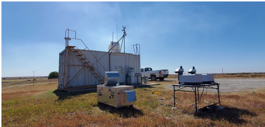
Figure 2.5: Deployment of Blanche and guest EM27/SUN instruments next to the ARM SGP TCCON station (white building) during the TCCON calibration campaign during October 17-19, 2022.
