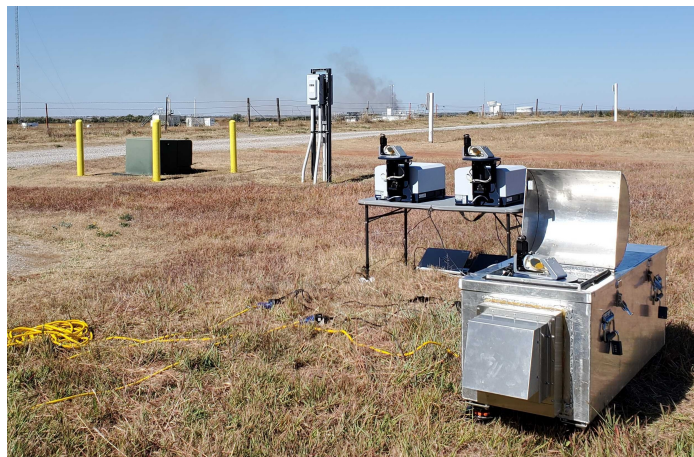
Figure 3.4: Blanche and the two guest EM27/SUN instruments at SGP on 10/17/22, where a plume of smoke blew into the viewing path of the instruments.
