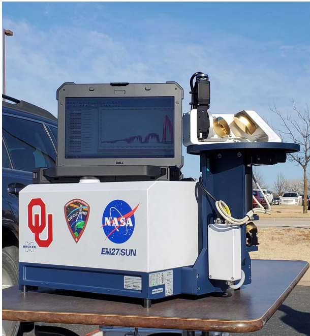
Figure 1.2: Blanche the EM27/SUN spectrometer, actively observing trace gases during a teaching demonstration
