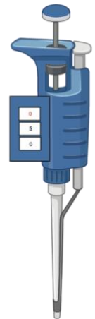
Figure 2-2 P1000 Micropipette with volume readout set to 050
