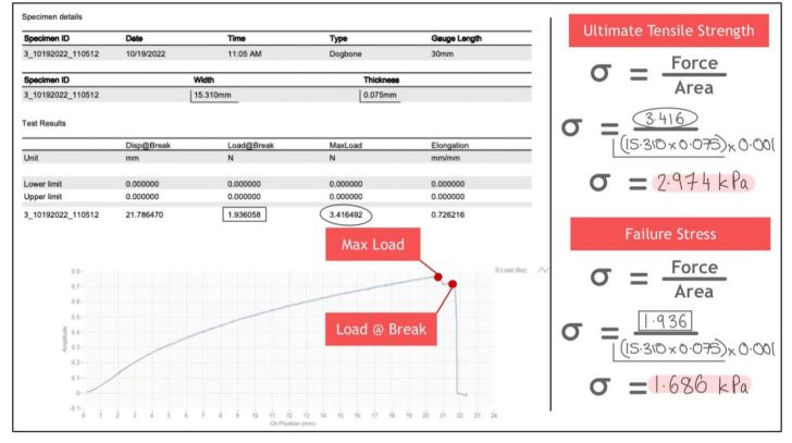
Figure 6-4 Detailed image showing extraction of data from pdf reports and calculation of Ultimate Tensile Strength and Failure Stress
