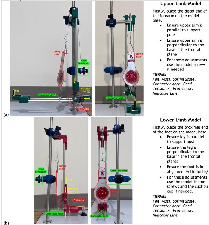
Figure 1-4 Labelled images and setup tips for the upper (a) and lower limb (b) Vernier musculoskeletal models.
