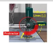
Figure 3-3 Labelled image showing 120 degrees of elbow flexion, guided with vernier model protractor and indicator lines.
