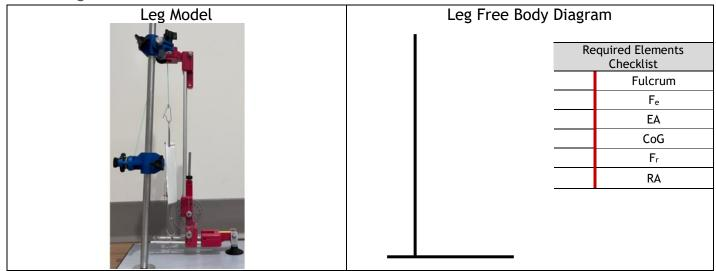
Figure 2-3 Mechanical leg model and leg free body diagram illustration.
