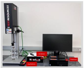
Figure 6-3 Newton TestResources Machine and accompanying computer. Labels show power button, job buttons and Newton
