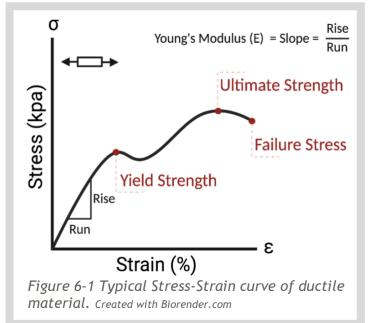
The slope of this line is called *Young's modulus* or modulus of elasticity. Therefore, in this linear elastic region we have  $\sigma = E\epsilon$ .
