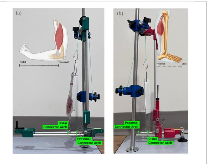
Figure 3-2 Labelled images illustrating the proximal and distal connector arches for the upper (a) and lower limb (b) Vernier musculoskeletal models. Some image components were created with BioRender.com
