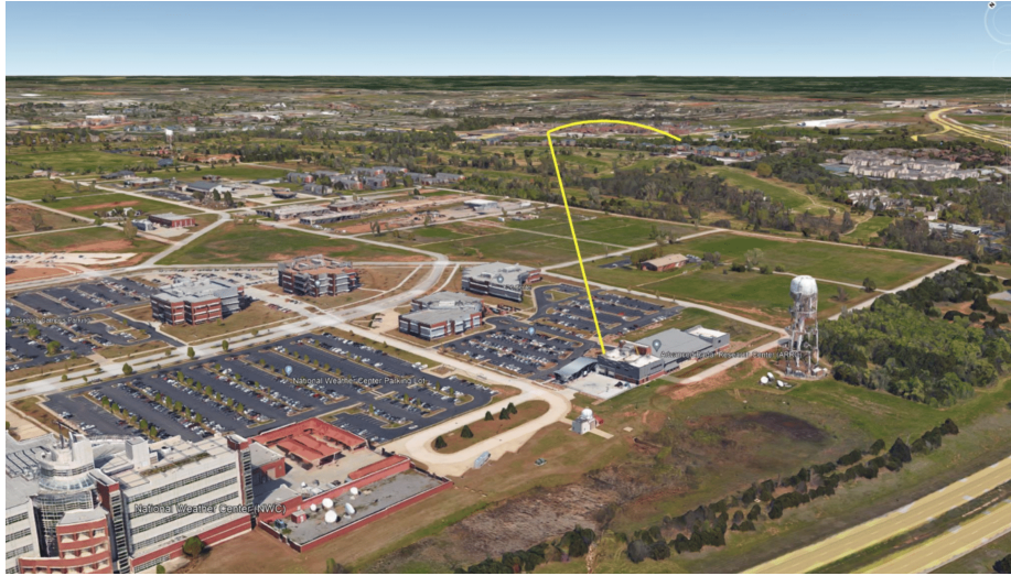
Figure 3.9: The spherical mission plan of the UAS as visualized in 3D. This is essential in verifying the mission safety and to ensure the UAS remains at a safe distance from all structures.
