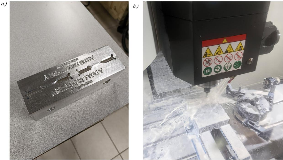
Figure 40: a.) Custom machined fixturing for machining off bottom layers of samples. b.) CNC machining of the samples using custom toolpaths and flood coolant to negate any chipping or stress concentrations.
