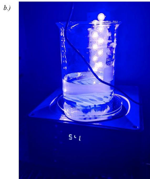
Figure 39: a.) Custom heated in-situ manufacturing enclosure system. b.) High-temperature underwater post-curing system.
