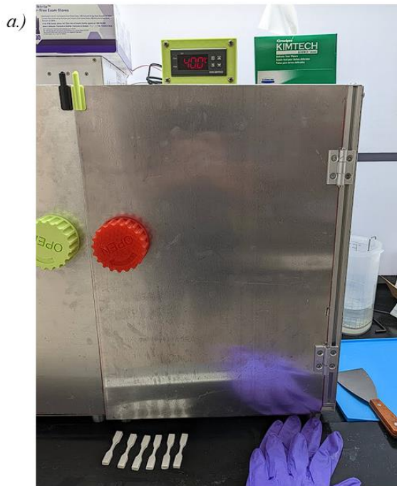
Figure 39: a.) Custom heated in-situ manufacturing enclosure system. b.) High-temperature underwater post-curing system.
