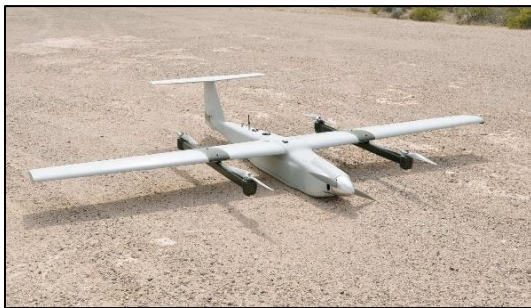
Figure 23: Aerovironment Jump-20 tractor quad plane
