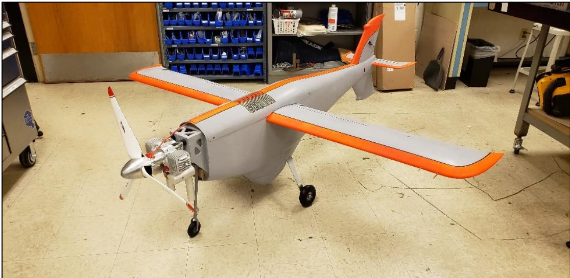
Figure 66: Locust controllable wing loading UAV [4]
