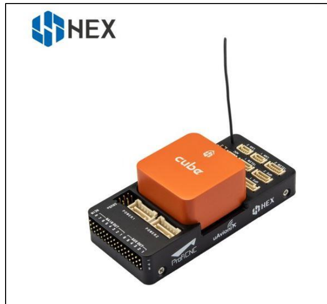
Figure 92: Cube Orange with standard carrier board
