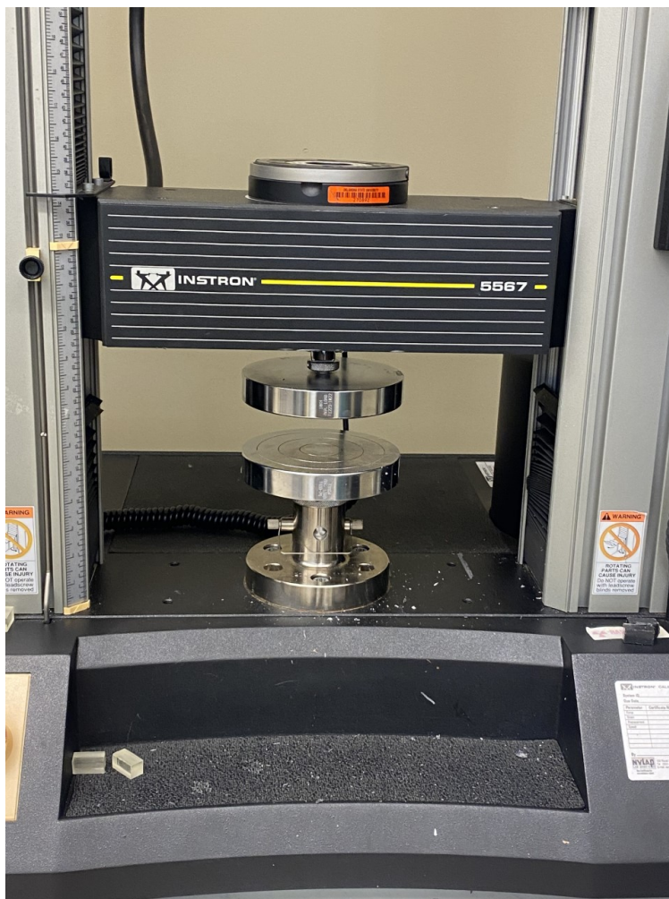
Figure 11: Instron 5567 equipped with a 10kN load cell
