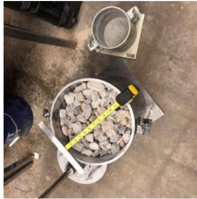
Figure 11: Picture Showing the Custom-Made Mold along with a Conventional 152.4-mm Diameter Proctor mold.
