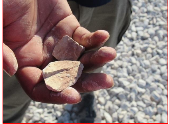
Breaking of the Aggregate Particle due to Over Compaction
