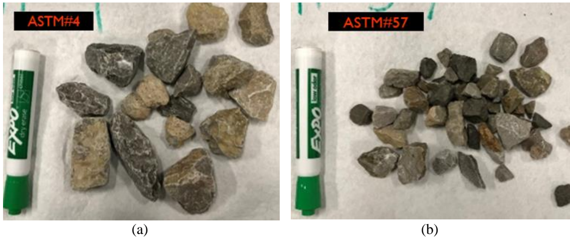
Figure 9: Particles from (a) ASTM # 4, and (b) ASTM # 57 Stockpiles
