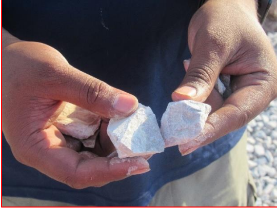
Breaking of the Aggregate Particle due to Over Compaction
