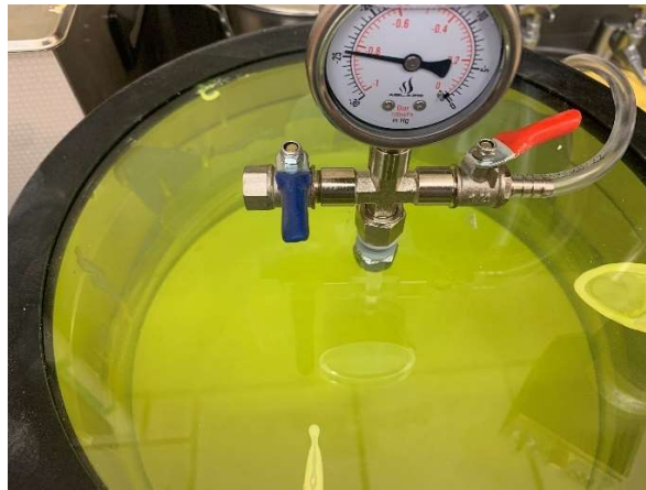
Figure 18. Displays the vacuum and lack of bubbles along the surface of Suspend-a-Slurry
