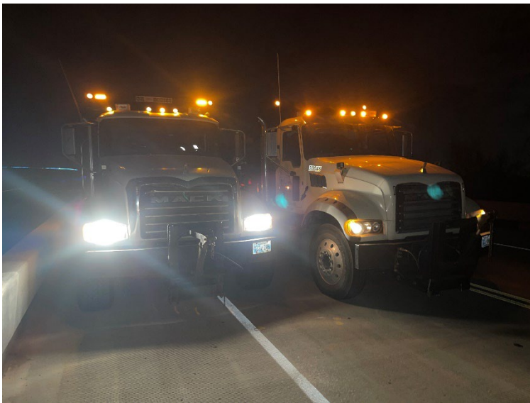
Figure 49: Truck configuration 3 for static load testing.
