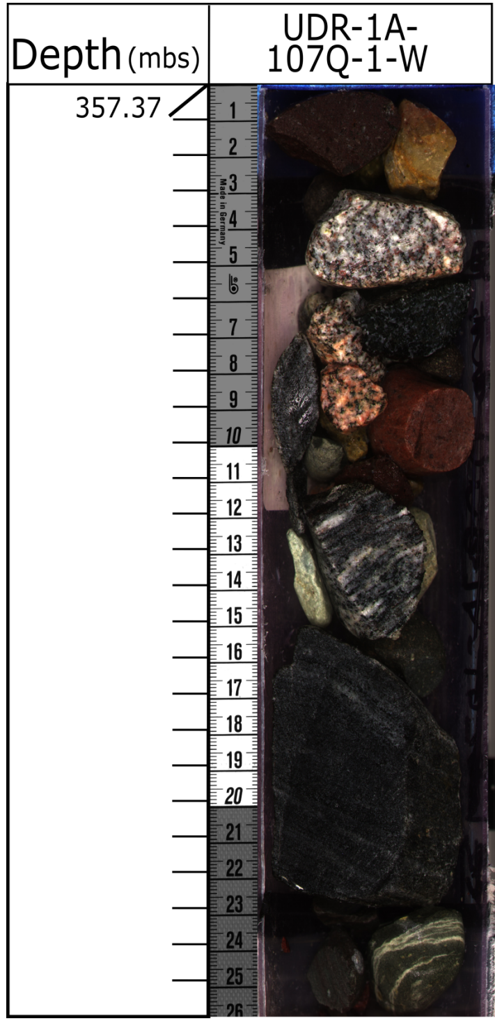
Figure 5: Section of the (inferred) ancestral Gunnison Gravels showing various (mostly basement) lithologies. The presence of intermediate volcanics (andesite) leads to the interpretation of these gravels originating from the Gunnison River.
