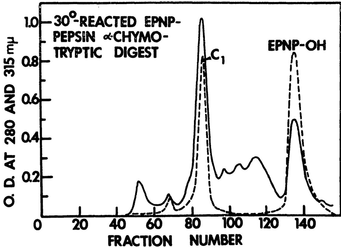
Fig. 7 - Chromatographic patterns of peptides from  $L$ -chymotryptic digest of  $30^{\circ}$ -reacted EPNP-pepsin. The solid line represents optical density at 280 nm and the broken line represents the optical density at 315 nm.
