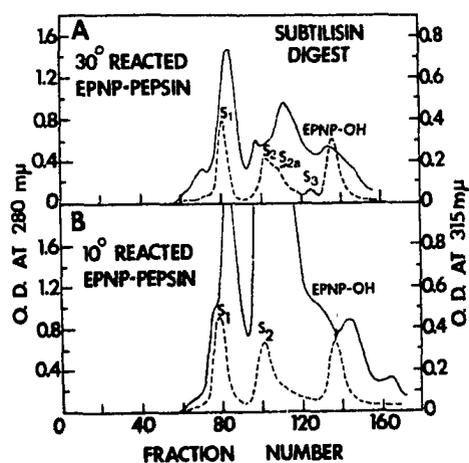
Fig. 3 - Chromatographic patterns of peptides from subtilisin digest of EPNP-pepsin inactivated at 30°(A) and at 10°(B) on a column of Sephadex G-25. The solid line represents optical density at 280 nm and the broken line represents optical density at 315 nm.
