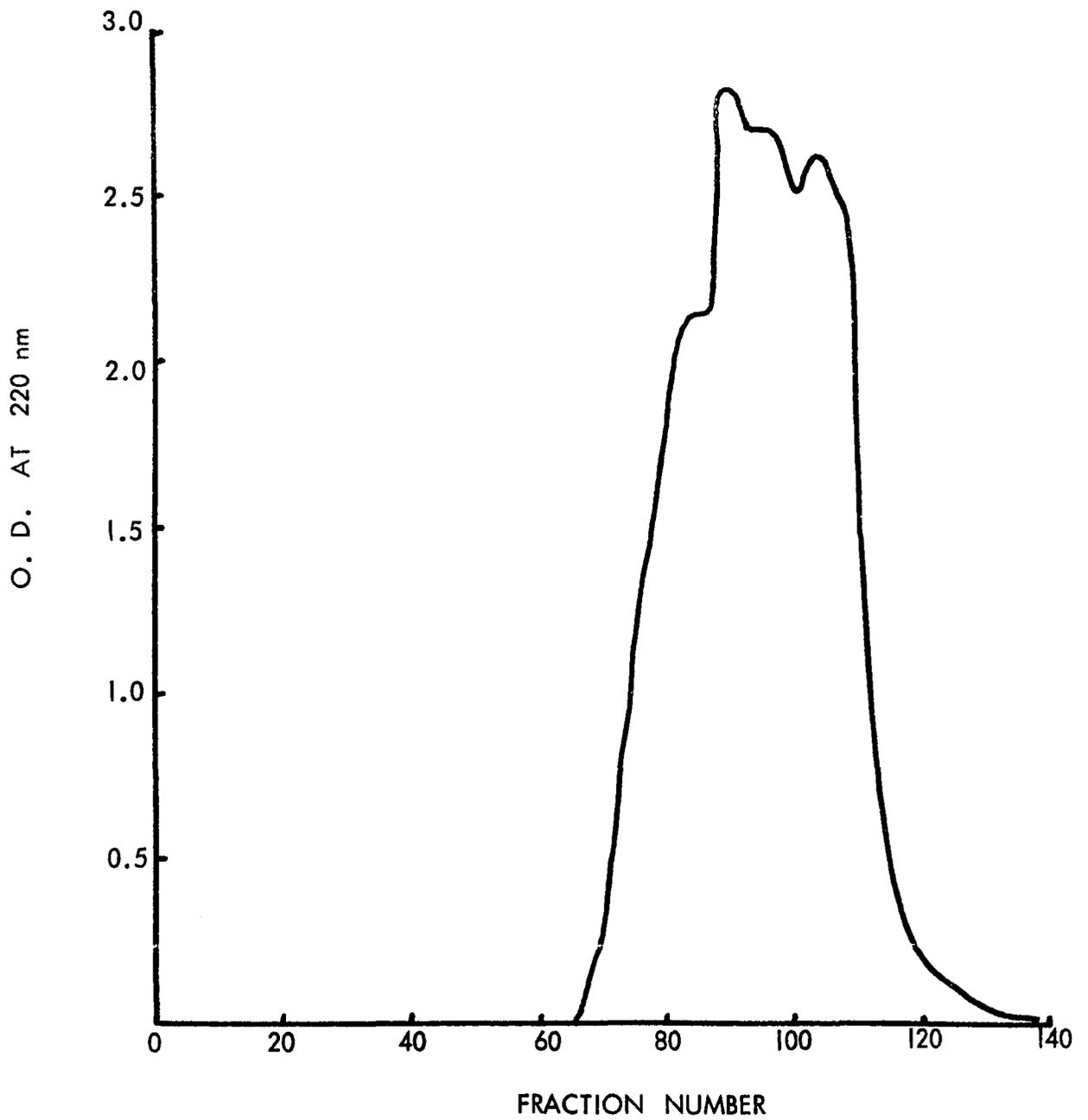
Fig. 17 - Chromatographic patterns of peptides from papain digest of CB5 on a column of Sephadex G-25. Each fraction contained 10 ml.
