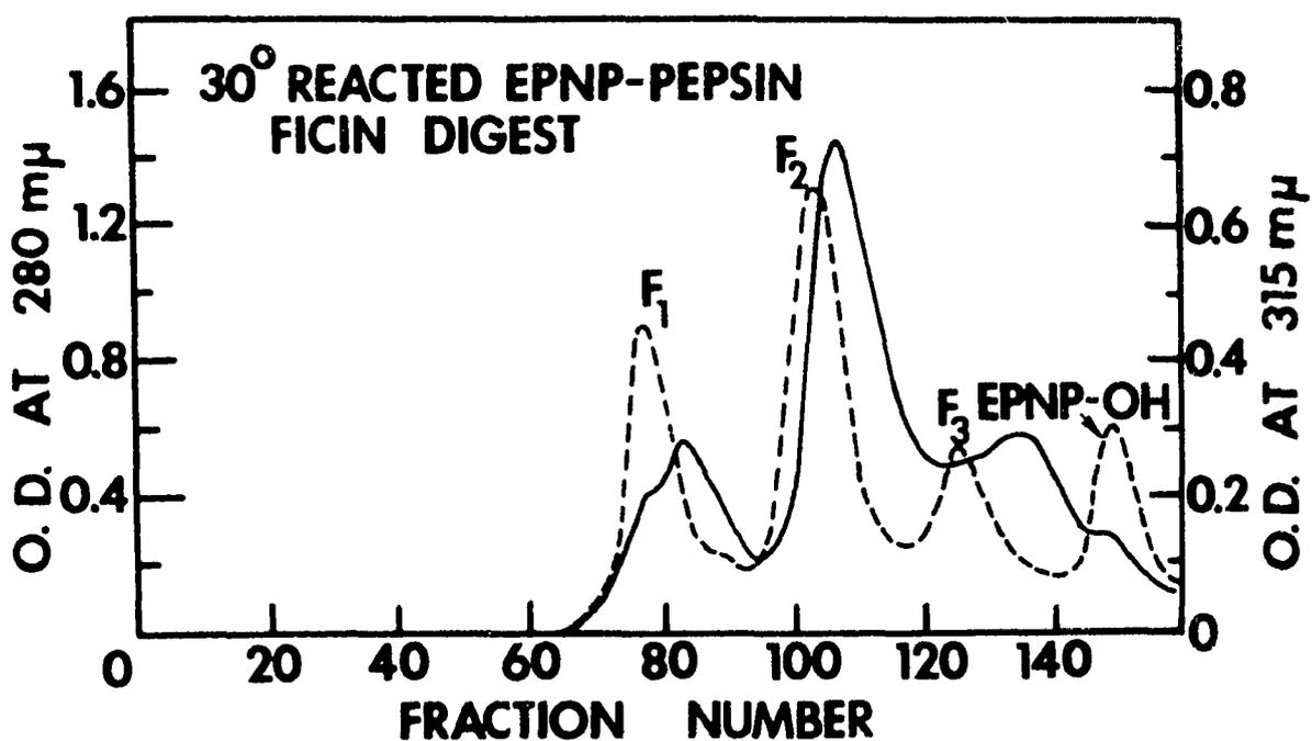
Fig. 5 - Chromatographic patterns of peptides from ficin digest of 30°-reacted EPNP-pepsin. The solid line represents optical density at 280 nm and the broken line represents the optical density at 315 nm.
