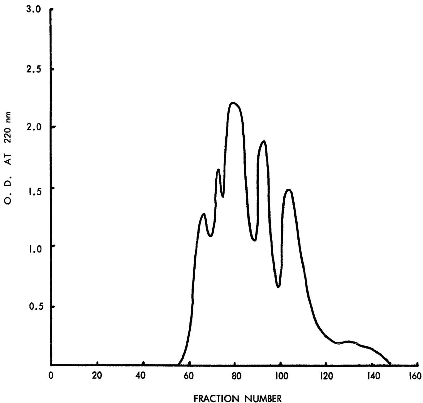
Fig. 15 - Chromatographic patterns of peptides from thermolysin digest of CB5 on a column of Sephadex G-25. Each fraction contained 10 ml.
