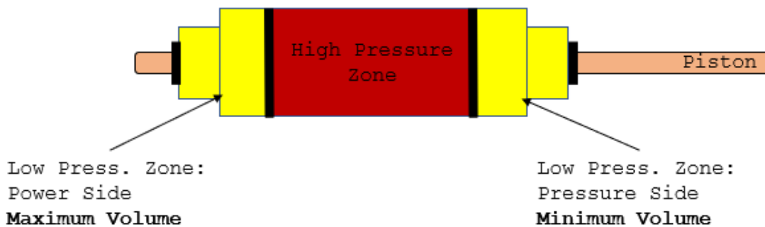
Figure 34: Piston in Far-Right Position
