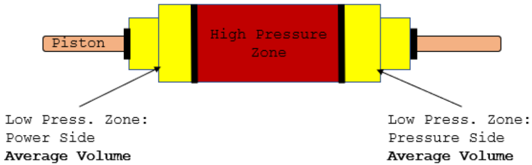
Figure 32: Piston in Neutral Position
