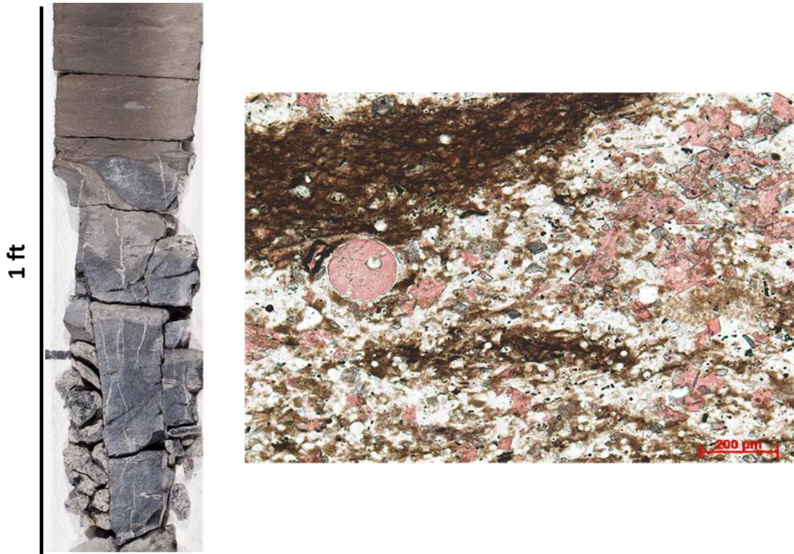
Figure 51. Major stratigraphic boundary in core. Left image is a core photograph of a diagenetically altered chert bed sharply overlain by mudstone and represents a disconformity at the Osagean-Meramecian boundary. Chert clasts are highly fractured, and the matrix between clasts is composed of dolomite and clay. Right image is a thin section photomicrograph containing spicules, and other microbioclastic debris and microbioclastic ghosts. Multiple episodes of cementation include calcite, chert, and dolomite.
