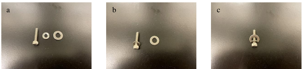
Figure H6. (a) 8-32 screw and two sizes of washers for lift stage assembly while (b) first small and then (c) big washer inserted to the screw.
