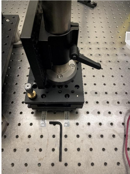
Figure H2. Removal of mounting post for battery measurements
