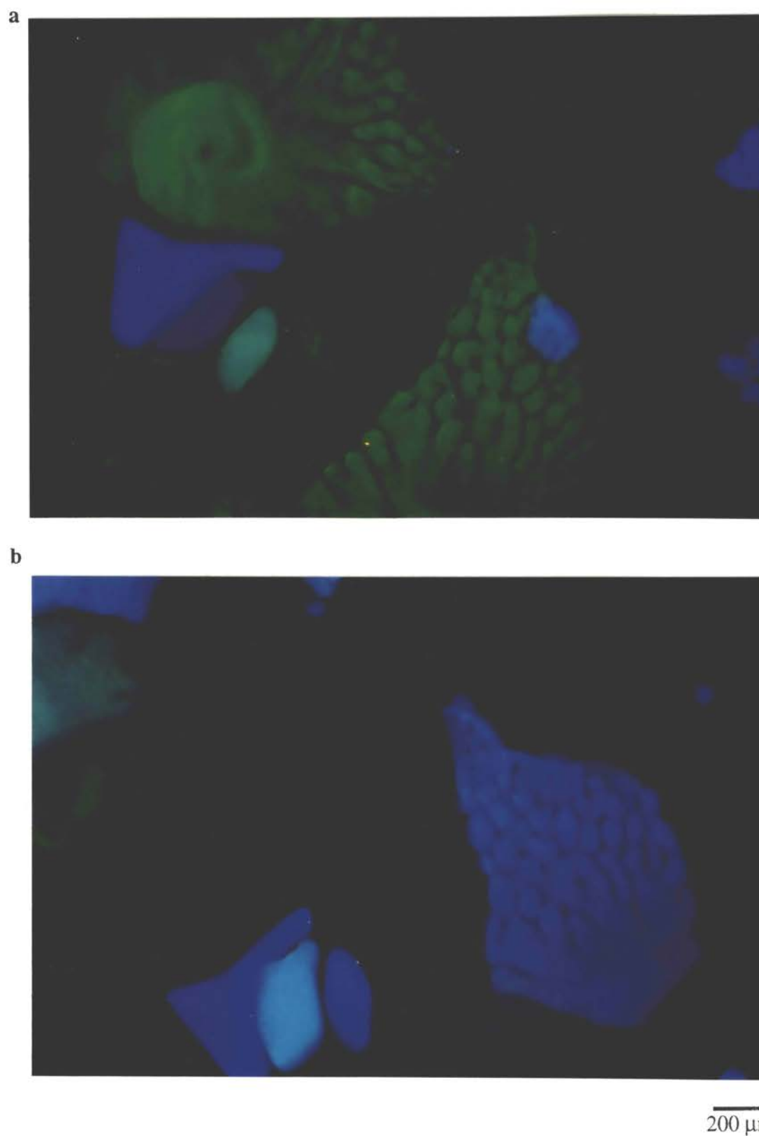
Figure 15. Polarizing microscope images of a 35 wt % 152 nm TPM-silica in MMA with incident light normal to the cell plane and at \beta -angle (a) 0, and (b) 30°.
