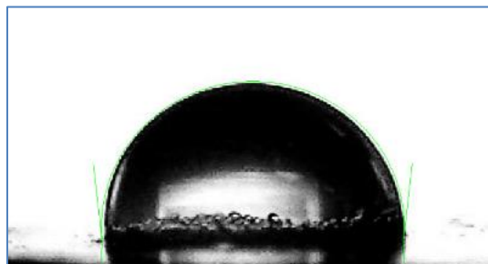
Figure 6.5. The picture of the water droplet on the GO-POSS-NH 2 surface
