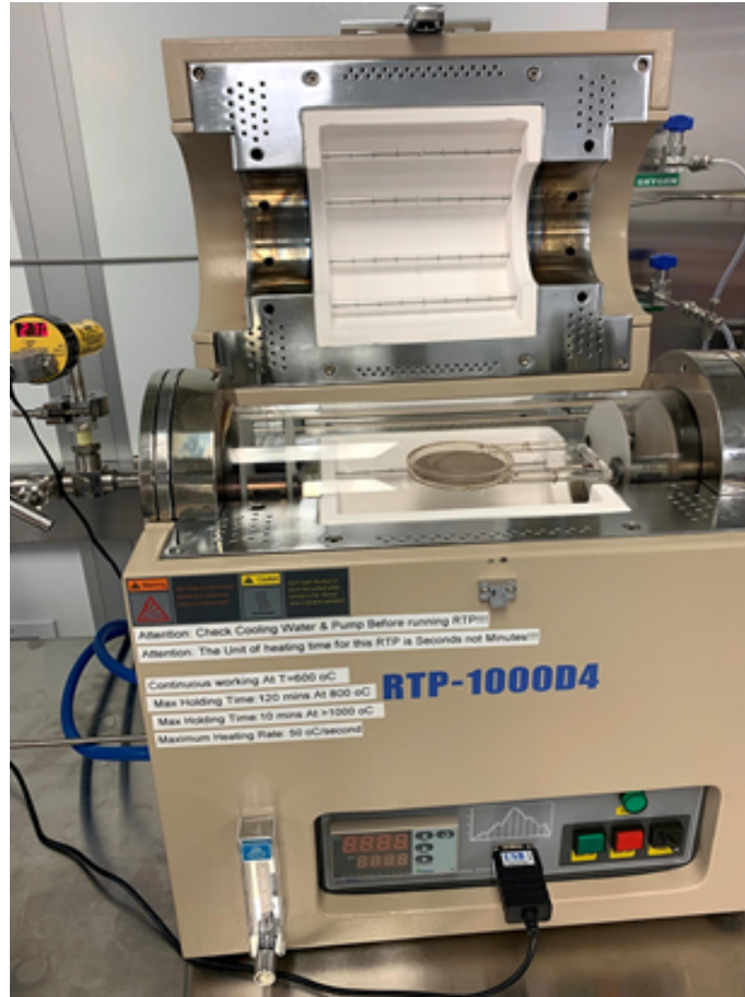
Figure 4.2: RTP-1000D4 by MTI rapid thermal annealer.
