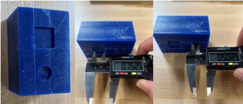
Figure 5.6: Measurements of Pockets
