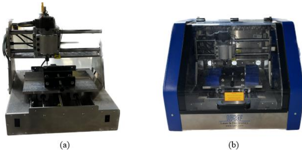
Figure 5.1: (a) Completed CNC Milling Router and (b) CNC Milling Router with Covers
