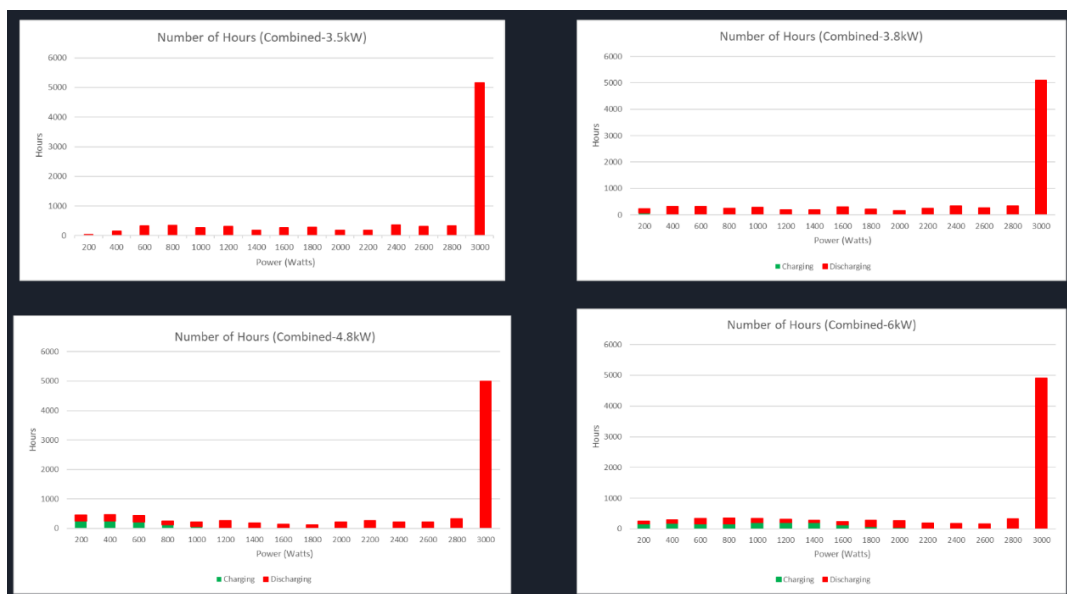
Figure 4.3j: Number of Hours the Solar is Charging and Discharging
