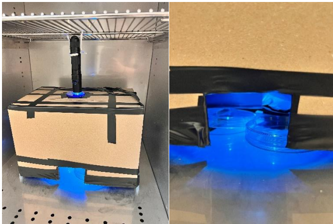
Figure 3 Phototactic movement set up for N. alkalilacustris sp using the ‘blue circle’ filter and the Fenix UC35 V2.0 1000 Lumen Rechargeable Tactical Flashlight with LumenTac Organizer on the 150 lumen setting. The box is lined with black paper to eliminate reflection of light outside the desired circular location.
