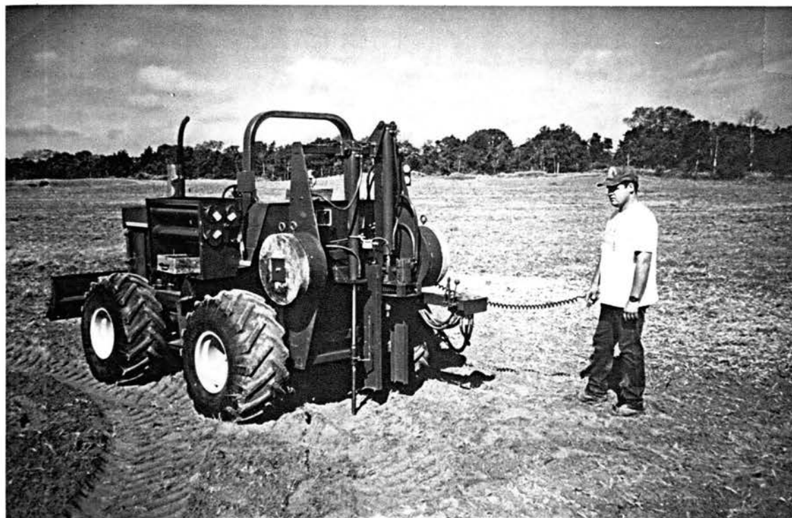
Figure 18: Penetrometer rig in use at Coyle test site. Auger sampling device is to the right of the penetrometer push cylinder.
