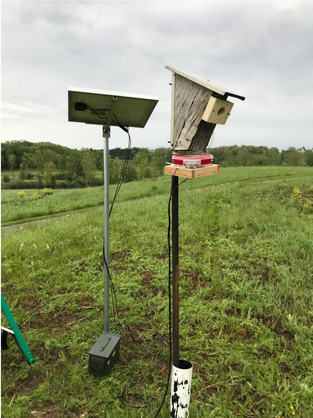
Figure 1.1. Radio frequency identification (RFID) reader and external speaker setup. The RFID readers were retrofitted onto existing nest boxes by placing the readers in plastic containers and placing the containers on a wooden shelf. RFID antennas were held in place using entrance guards.
