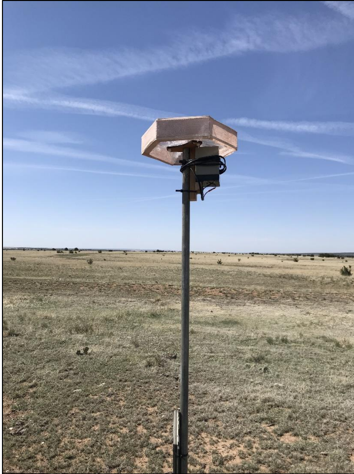
Figure 3.3. HEXEAR case with AudioMoth automated recording unit. To reduce wind noise, we wrapped each HEXEAR in gauze as a windscreen. Each HEXEAR was placed on top of a 1.27 cm diameter conduit pole to increase the recording coverage.
