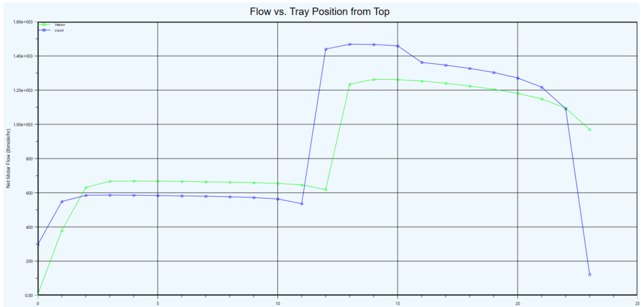
Figure 8. Vapor/Liquid Traffic Per Stage Profile from HYSYS
