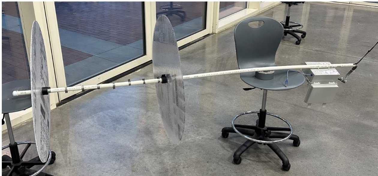
Image 10: Baffle Shaft Setup with Temperature Sensors and Instrumentation Box
