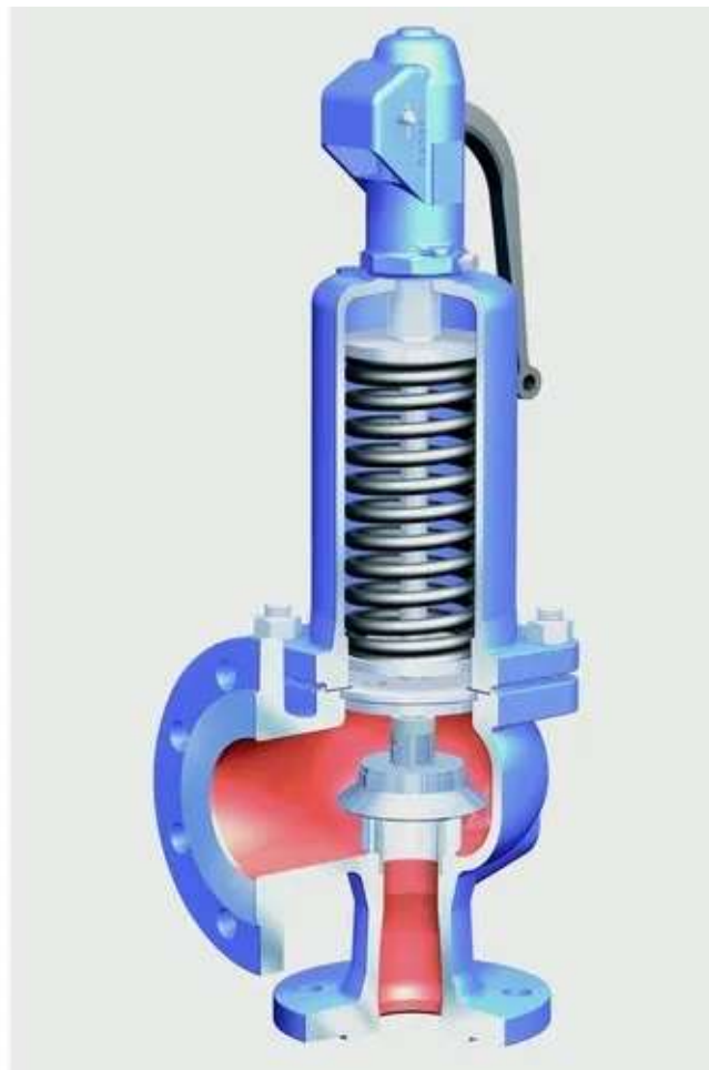
Figure 7: Conventional Relief Valve [9]
