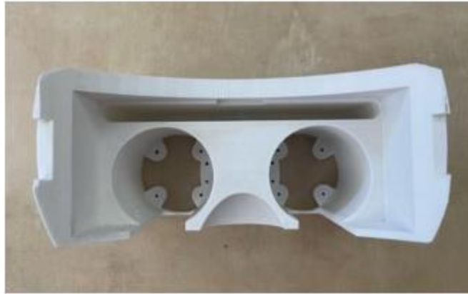
Figure 2.1 Prototype I. Prototype of the 3D printed video-oculography headset without the cameras, Raspberry Pi, and smartphone attached. The two eye holes are intended for the cameras, the top hole is for the smartphone, and the Raspberry Pi will be secured on top. The strap mounts are located on the side and are broken.
