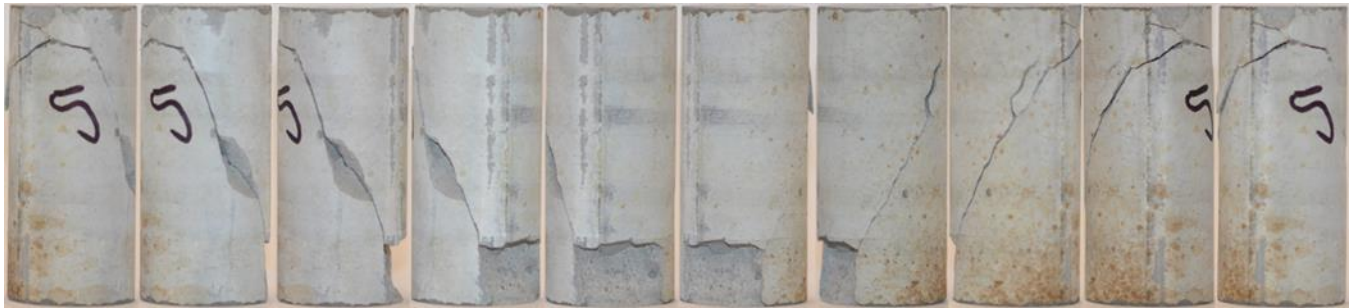
Figure A.5. Sample 5 sheared at 15 MPa.
