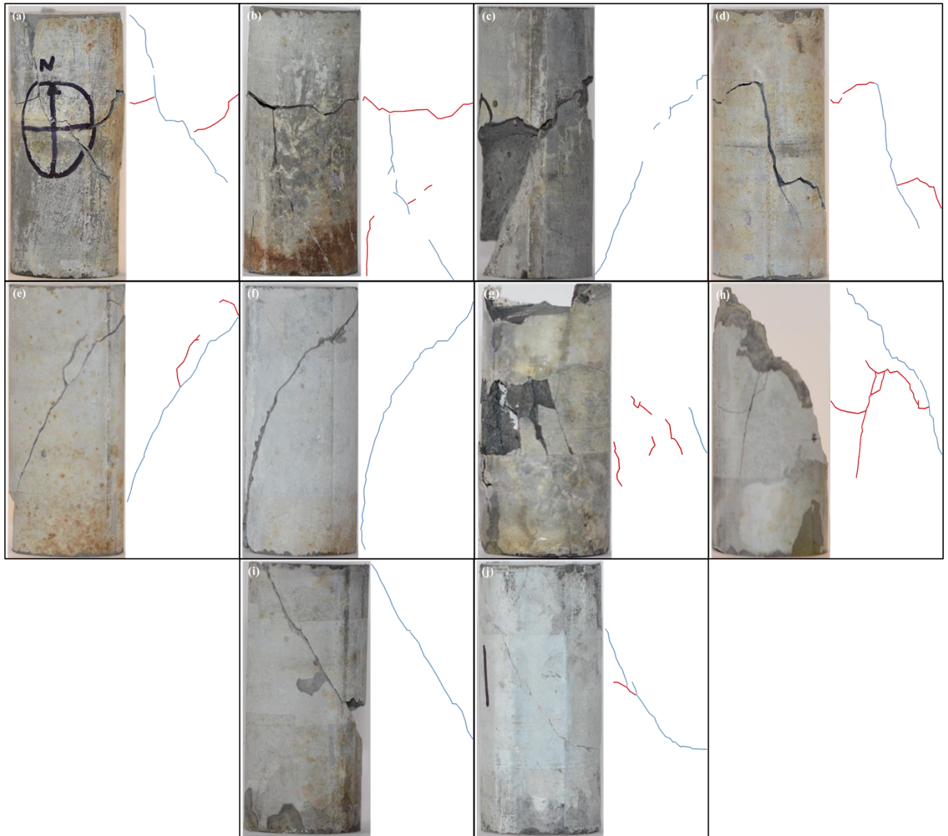
Figure 5.7. Fracture angle determination for a) Sample 1; b) Sample 2; c) Sample 3; d) Sample 4; e) Sample 5; f) Sample 6; g) Sample 7; h) Sample 8; i) Sample 9; j) Sample 10.
