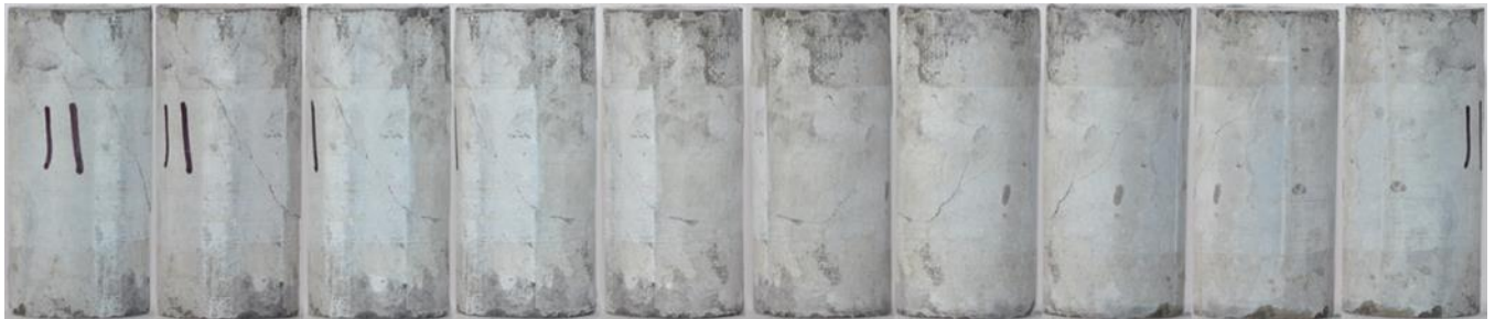
Figure A.10. Sample 10 sheared at 30 MPa.
