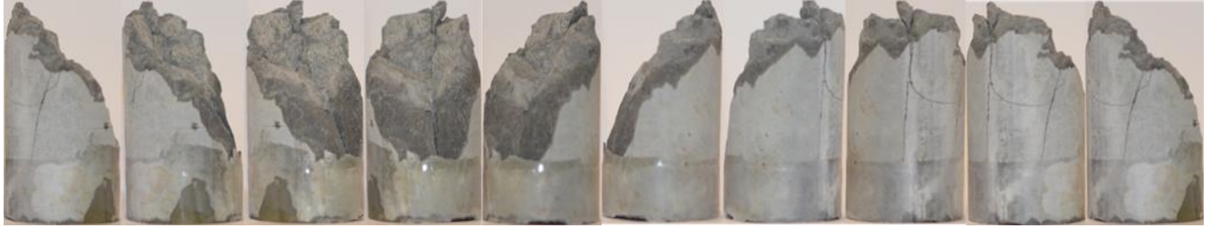
Figure A.8. Sample 8 sheared at 30 MPa.
