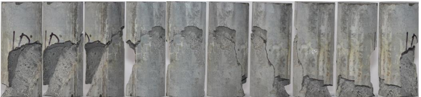
Figure A.2. Sample 2 sheared at 5 MPa.
