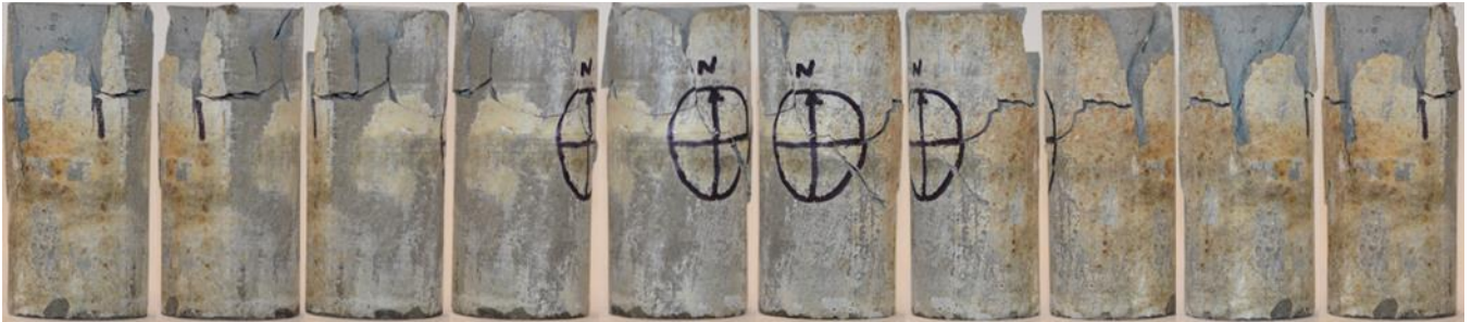
Figure A.1. Sample 1 sheared at 5 MPa.
