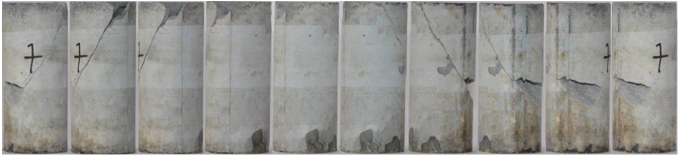
Figure A.9. Sample 9 sheared at 30 MPa.
