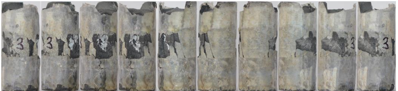
Figure A.7. Sample 7 sheared at 30 MPa.
