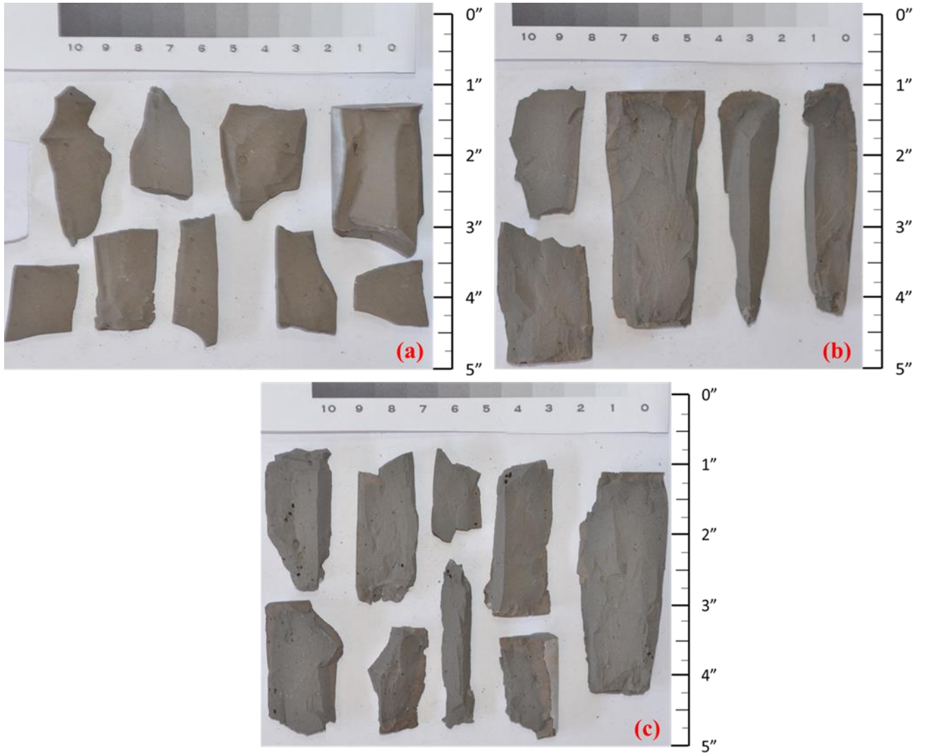
Figure D.17. 25% submicron case sample cured for 28-days (a) 1; (b) 2; (c) 3 after UCS testing.
