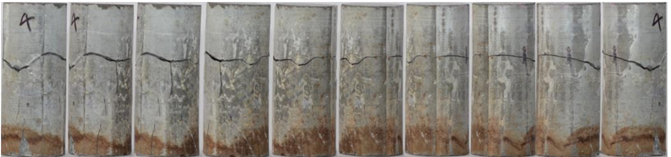
Figure A.1. Sample 1 sheared at 5 MPa.
