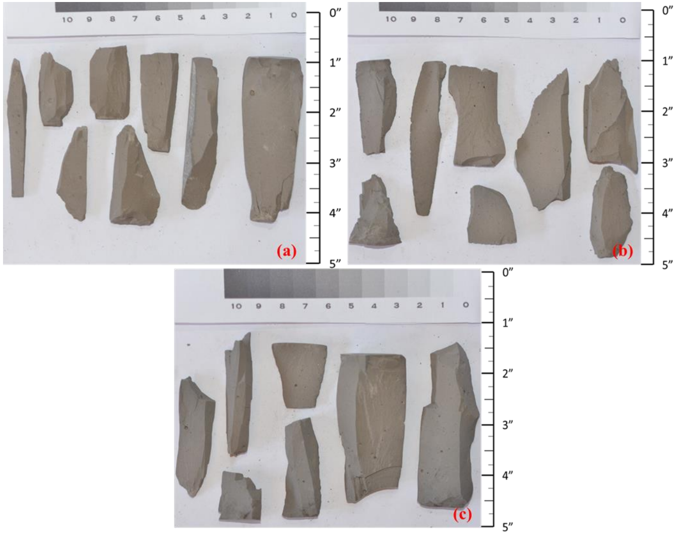
Figure D.16. 15% submicron case sample cured for 28-days (a) 1; (b) 2; (c) 3 after UCS testing.
