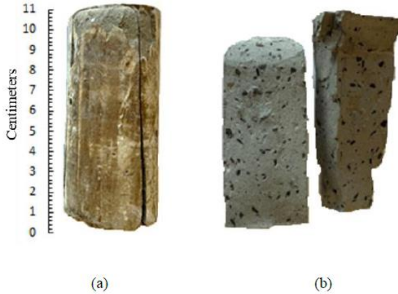
Figure 6.3. (a) A 5% submicron cement sample after UCS testing. (b) A 10% millimeter sample after UCS testing.
