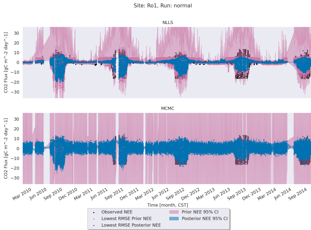
Figure 3.9: A time series plot of NEE observations (black), VPRM NEE with parameters from the parameter sets corresponding to the lowest RMSE and 95% confidence interval of the prior RMSE distribution (red), and VPRM NEE using parameter sets corresponding to the lowest RMSE and 95% confidence interval of the posterior RMSE distribution (blue), for the STIR non-linear least squares (top panel) and the MCMC (bottom panel) parameter fitting techniques fitting the whole dataset simultaneously for the Ro1 AmeriFlux site.
