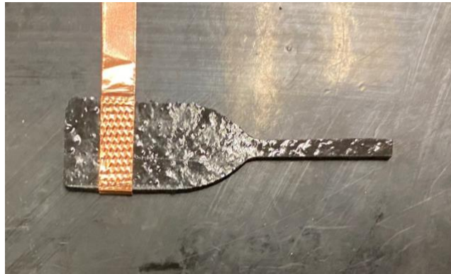
Figure 9: Sample with copper tape attached
