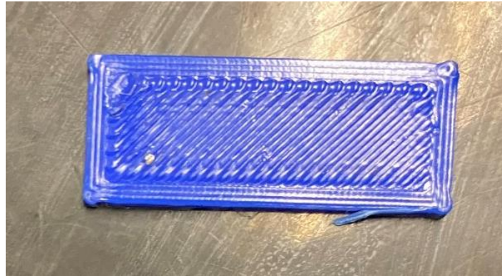
Figure 13: 3D Printed rectangular die
