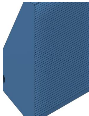
Figure 20: Close view of textured surface to increase grip
