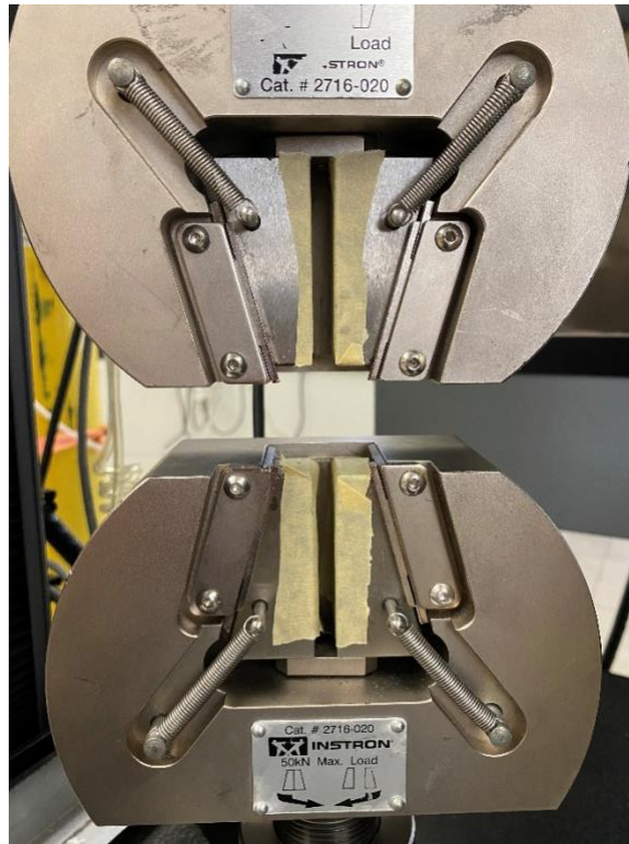
Figure 18: Paper tape applied to the metal jaws of the Instron machine
