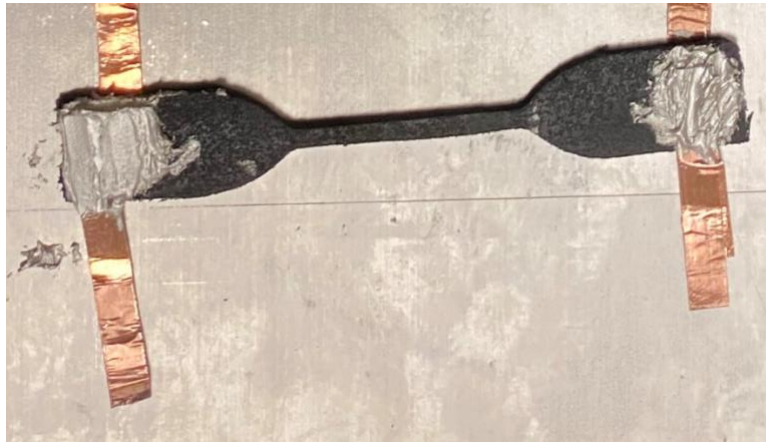
Figure 11: Rectangular samples with epoxied copper electrodes
