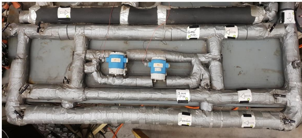
Figure 3.2: Rheology testing section of the experimental setup
