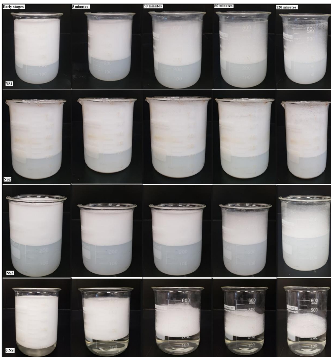
Figure 4.10: Image foam silica-nanoparticles dispersion (Top three rows) and pure surfactant foam dispersion (Bottom) overtime
