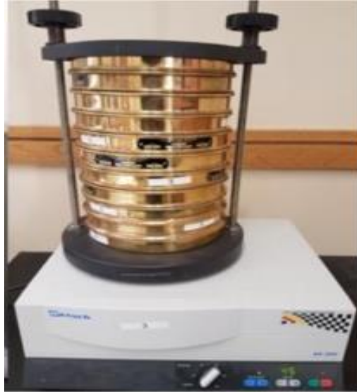
Figure 3.7: Sieve Analyzer used for determining the PSD for SMP and walnut LCM
