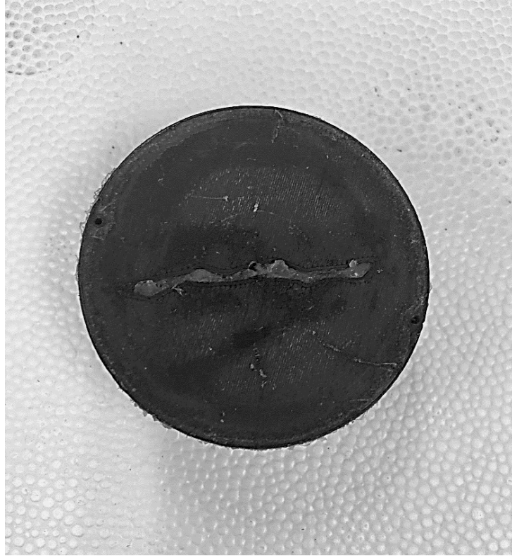
Figure 4.14: Sealed tapered fracture with PAM/PEI polymer mud at 150°C (302°F)
