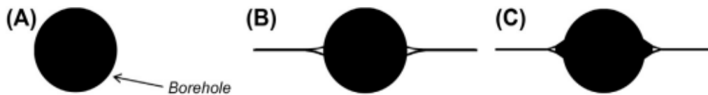
Figure 2.7: Initiation of a drilling-induced fracture: (A) before Initiation; (B) after the fracture has opened but mud invasion; (C) the fracture has opened and mud invasion in the fractured body.
