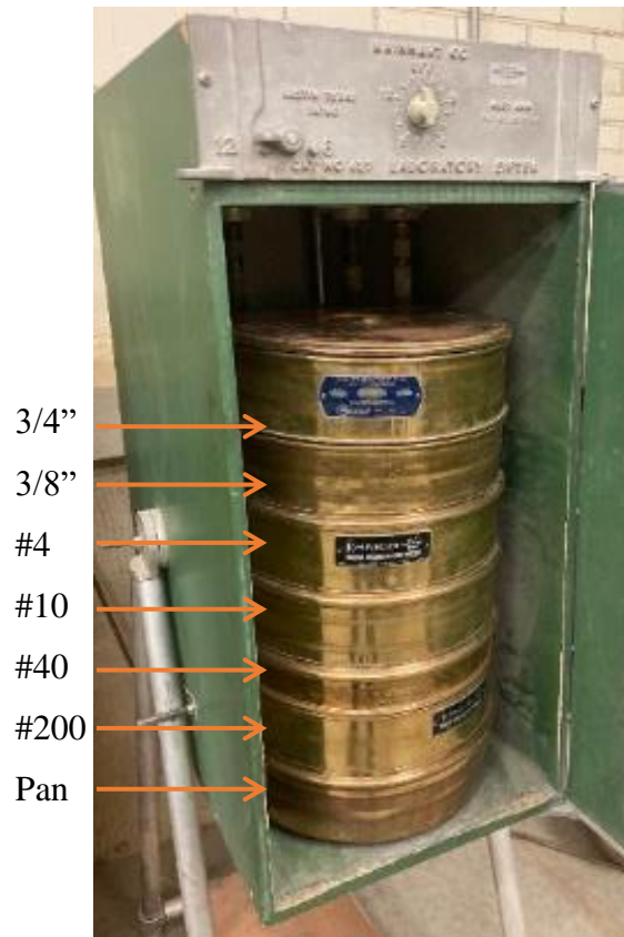
Figure 3-4: Mechanical sieving machine
