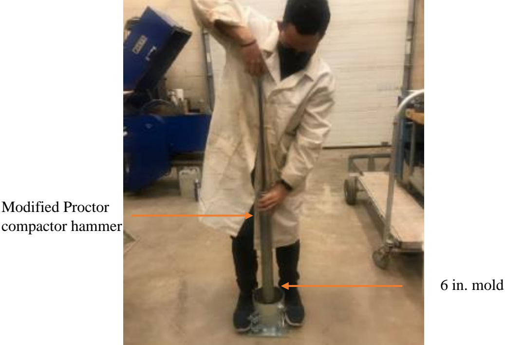
Figure 3-9: Modified Proctor test
