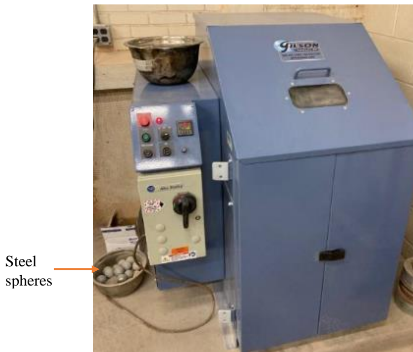
Figure 3-5: LA abrasion machine
