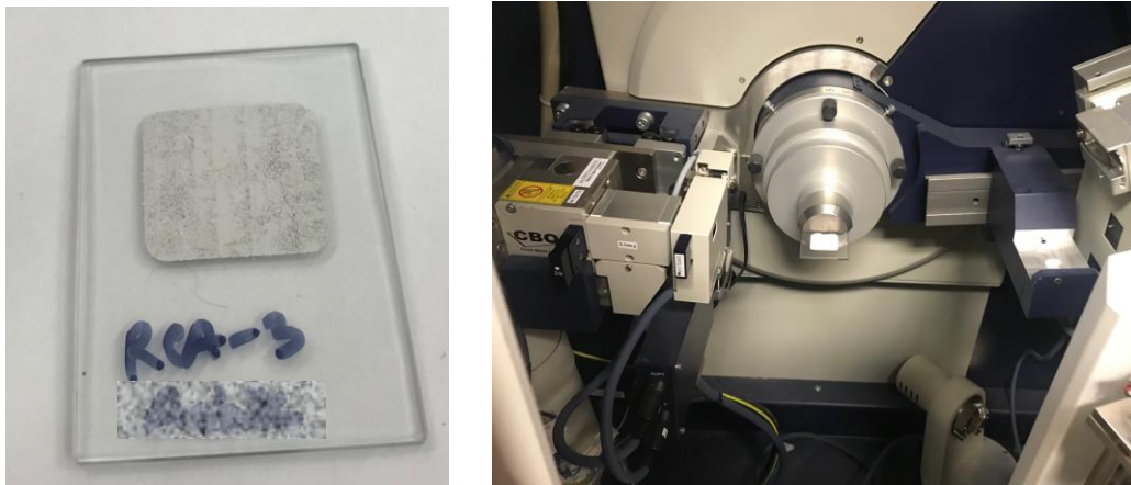
Figure 4-5: (a) Powder XRD sample and (b) XRD test setup
