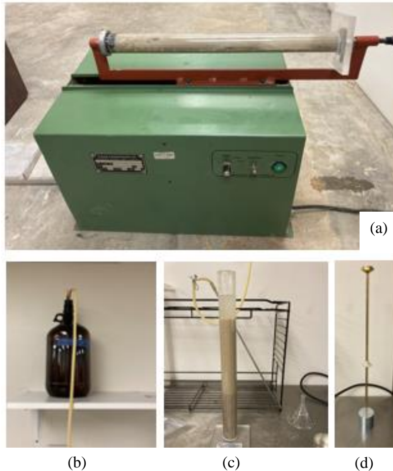
Figure 3-7: Durability of finer part; a) sand equivalent shaker; b) working solution; c) cylindrical tube; and d) weighted foot assembly
