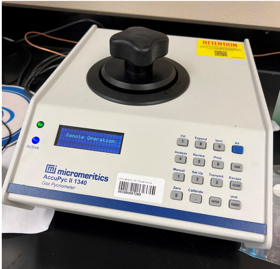
Figure 50: AccuPyc II 1340 Gas Pycnometer to Measure the Density Test Samples
