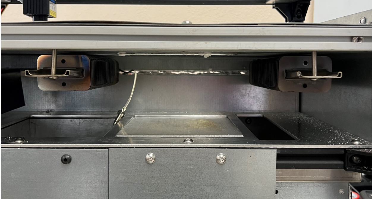
Figure 24: Heating Elements Installed in the Heat Chamber
