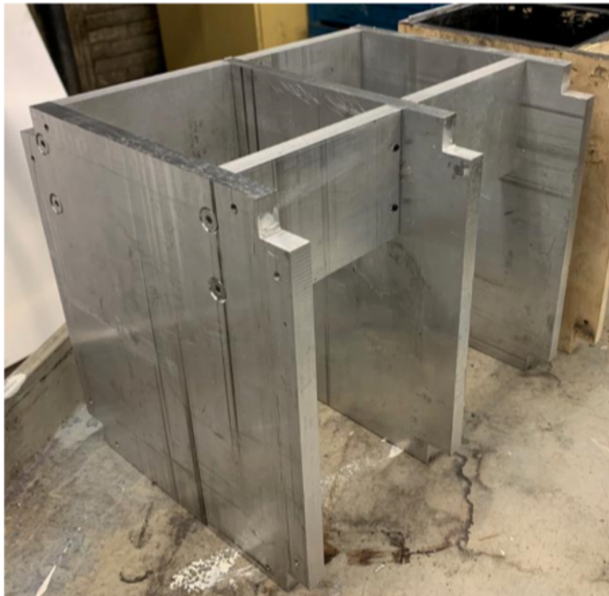
Figure 8: Piston Housing Manufactured out of T6061 Aluminum
