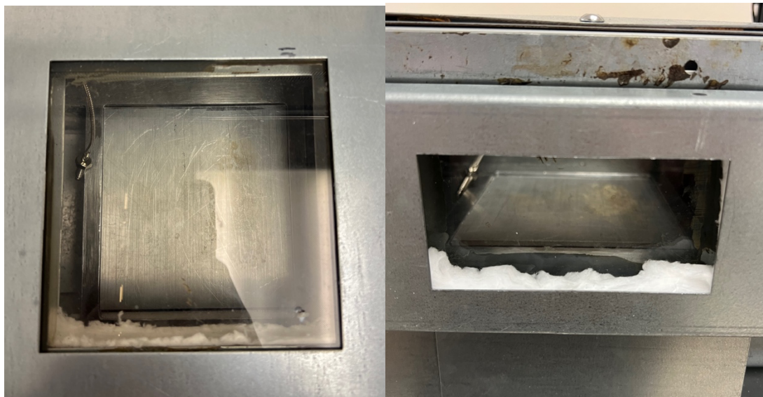
Figure 15: Heat Chamber Glass Viewing Windows
