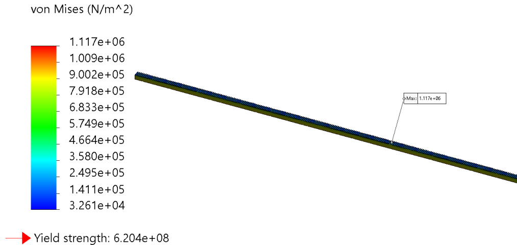
Figure 24: Stress on Rack from Gear
