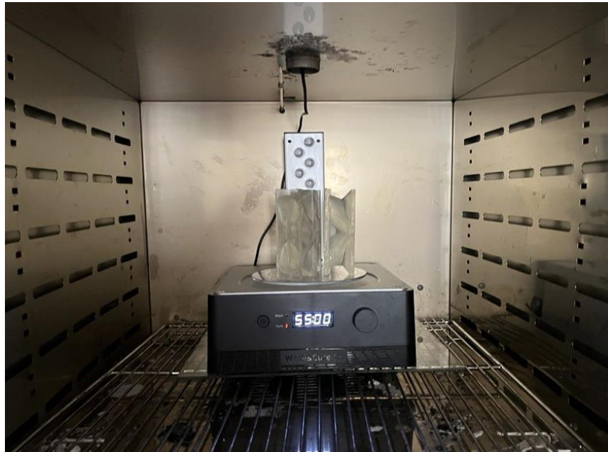
Figure 23: Curing and Heating Chamber for Resin Parts
