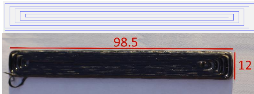
Figure 25: Specimen printing path and final part as used in tension and burnoff testing
