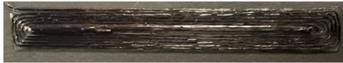
Figure 16: First successful specimen with long, straight lines printed using a flared needle
