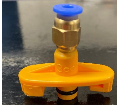
Figure 31: Pneumatic syringe cap with push-to-connect fitting
