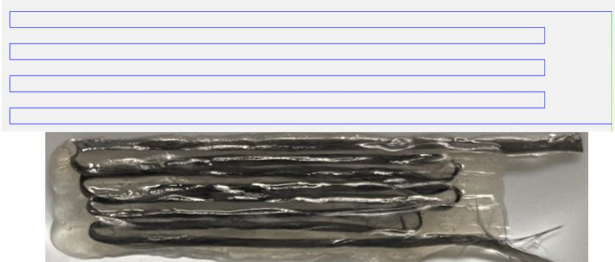
Figure 3: Earliest successful printed sample (below) using unmodified printer with its intended G-code path (above)
