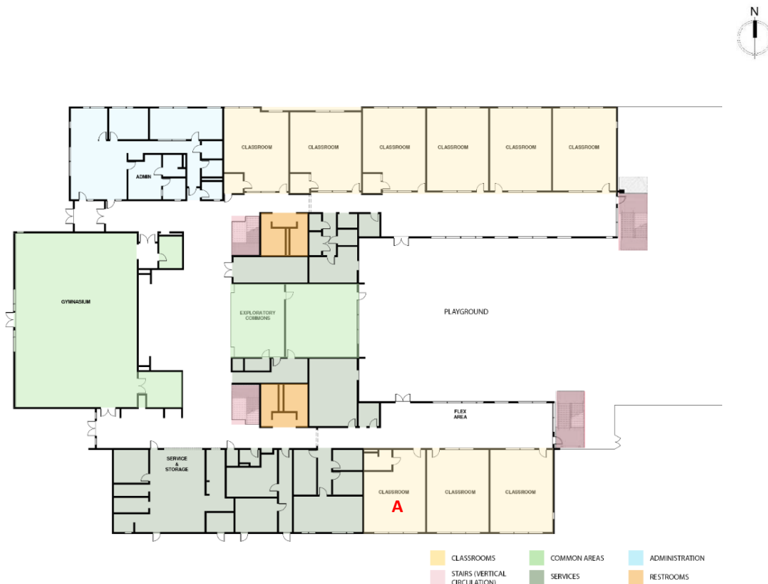
Figure 40. Browns Point Elementary School Zoning – 1st Floor (Design Credit: TCF Architecture / Drawn By: Author)
