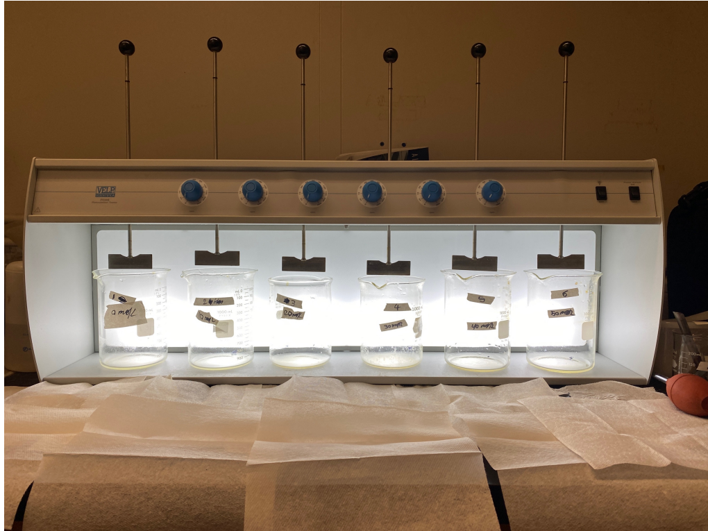
Figure 2. Jar Test Experimental Setup.
