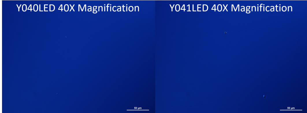
Figure 4.10: DIC imaging under 40 \times magnification for Y040LED (left) and Y041LED (right). Both structures have quite smooth surfaces, with few defects.
