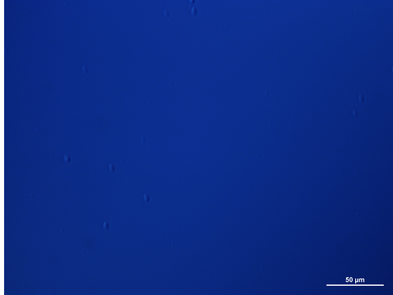
Figure 3.6: Example of typical oval hillock defects under 40X magnification in Y065V, an ICTPV structure taken in Nov. 2018.
