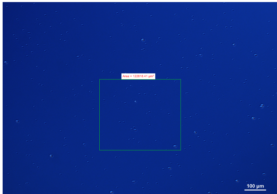
Figure 3.7: Example of a surface defect count showing about 45 defects in the traced out area on the surface of an ICPV structure (Y072V) taken at 10X magnification in April 2019.
