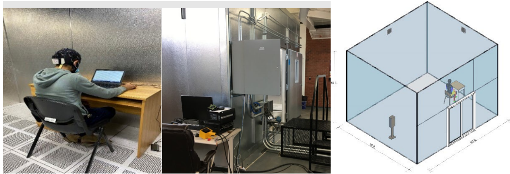
Figure 6.1 - OU environmental chamber: human subject inside the chamber; middle: chamber control and monitoring system right: Psychometric climate chamber showing experimental setup.
