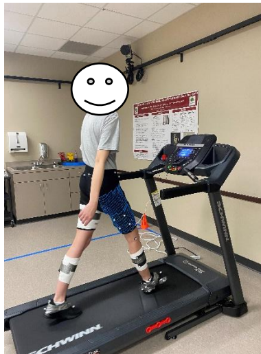
Figure 14. Participant undergoing the second walking warm-up prior to the overground walking trials. The participant walked at 3 MPH at 0° incline for five minutes.
