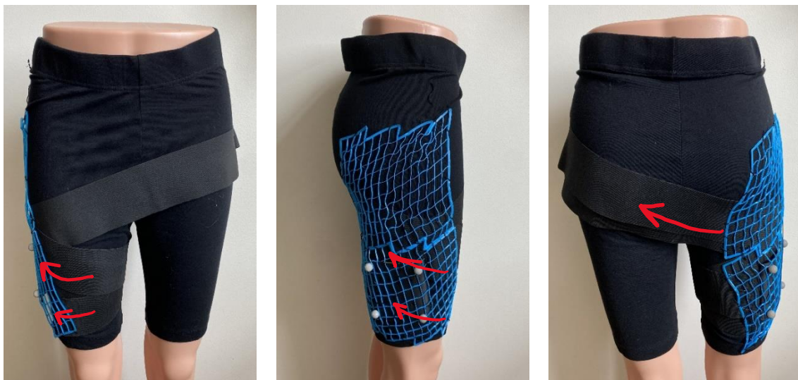
Figure 12. Final prototype of the brace. The direction of force applied by elastic is designated with arrows.
