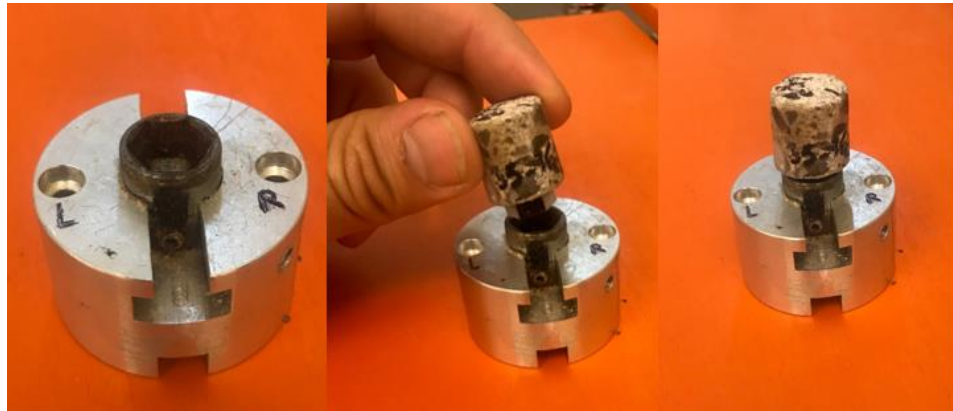
Figure 5-3.Ap. The designed stage for holding the sample
