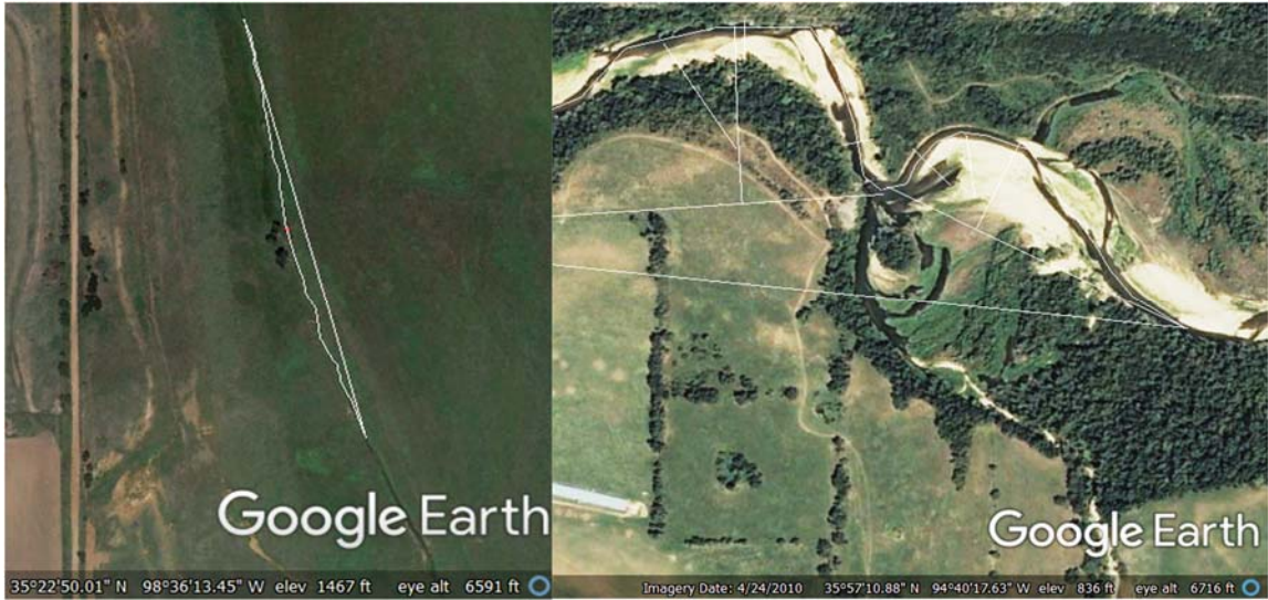
Figure 12: Meander measurements for a site in the Fort Cobb reservoir (left) and from Barren Fork (right). Notice that at a similar eye altitude (in bottom right corner of each picture) there is a significant difference in meandering. Google Earth cited the image on the right as coming from the U. S. Department of Agriculture, Farm Service Agency.
