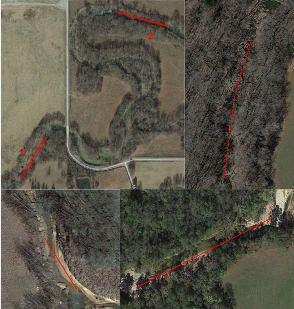
Figure 40: Google Earth images (various imagery dates) of all the validation reaches that failed the digital Channel Stability Index (CSI). Going clockwise starting in the top left corner: Fourche Maline, reach 1 & 2; Feather; Spring, reach 4; Sandy, reach 1. Note how these reaches are relatively straight.
