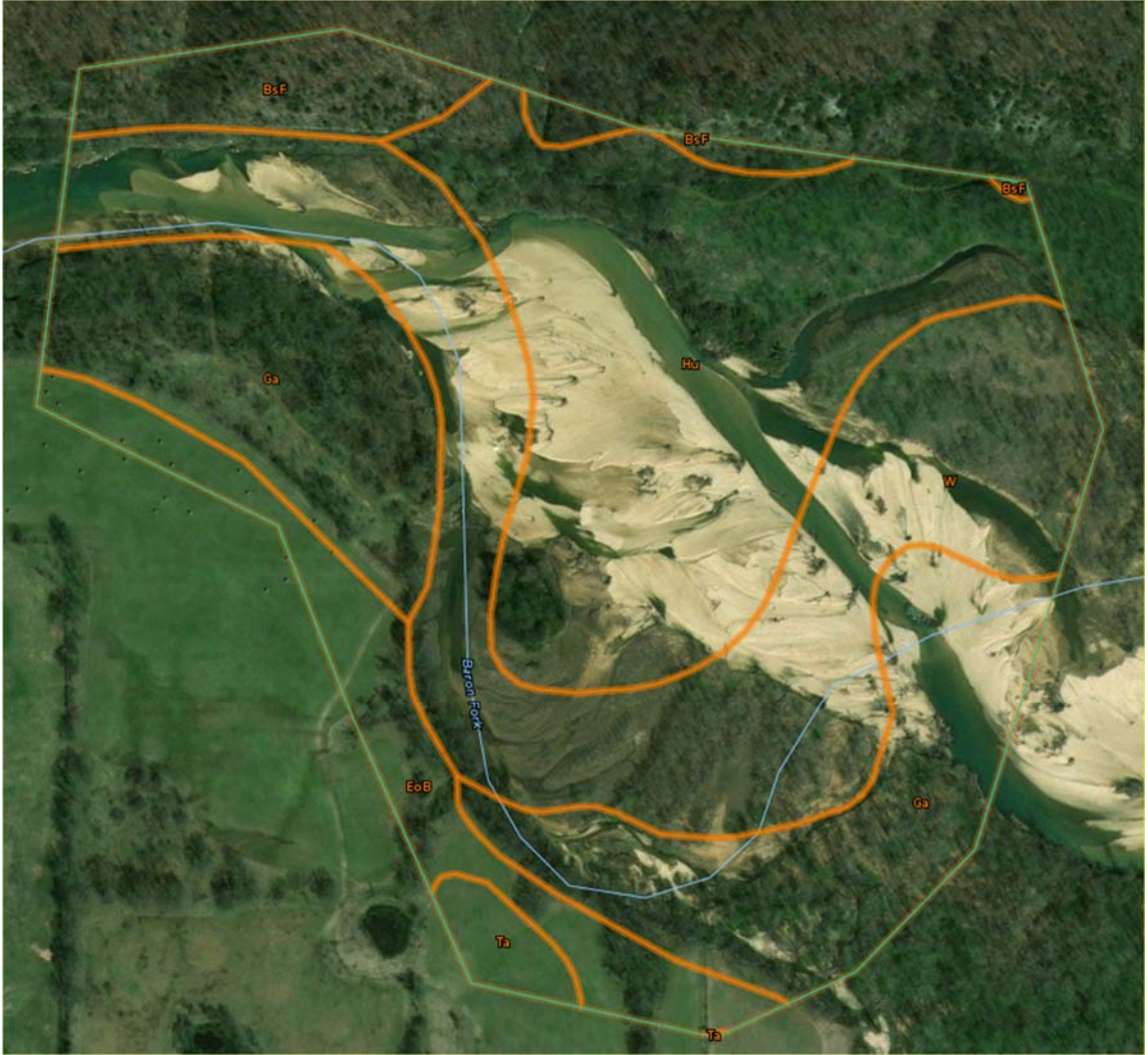
Figure 7: Example of Web Soil Survey map. Note how the stream, denoted by a W in the soil map, does not line up with the course of the stream in the background imagery.
