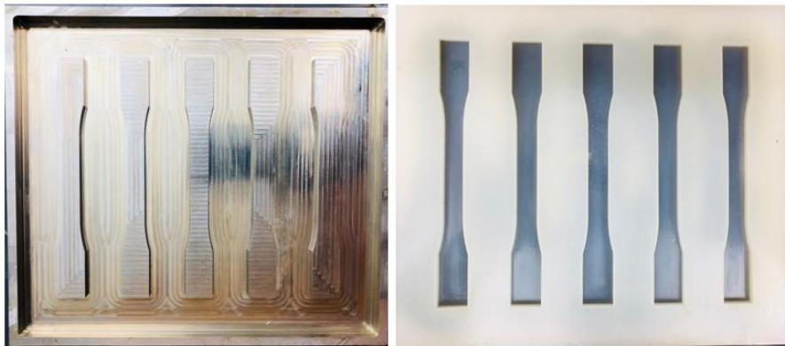
Figure 8 Mold negative and silicone mold used to prepare samples for tensile testing on Instron
