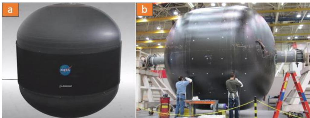
Figure 1 Composite Cryogenic Tanks developed by NASA and BOEING a) 2.4m diameter tank b) 5.5m diameter tank.
